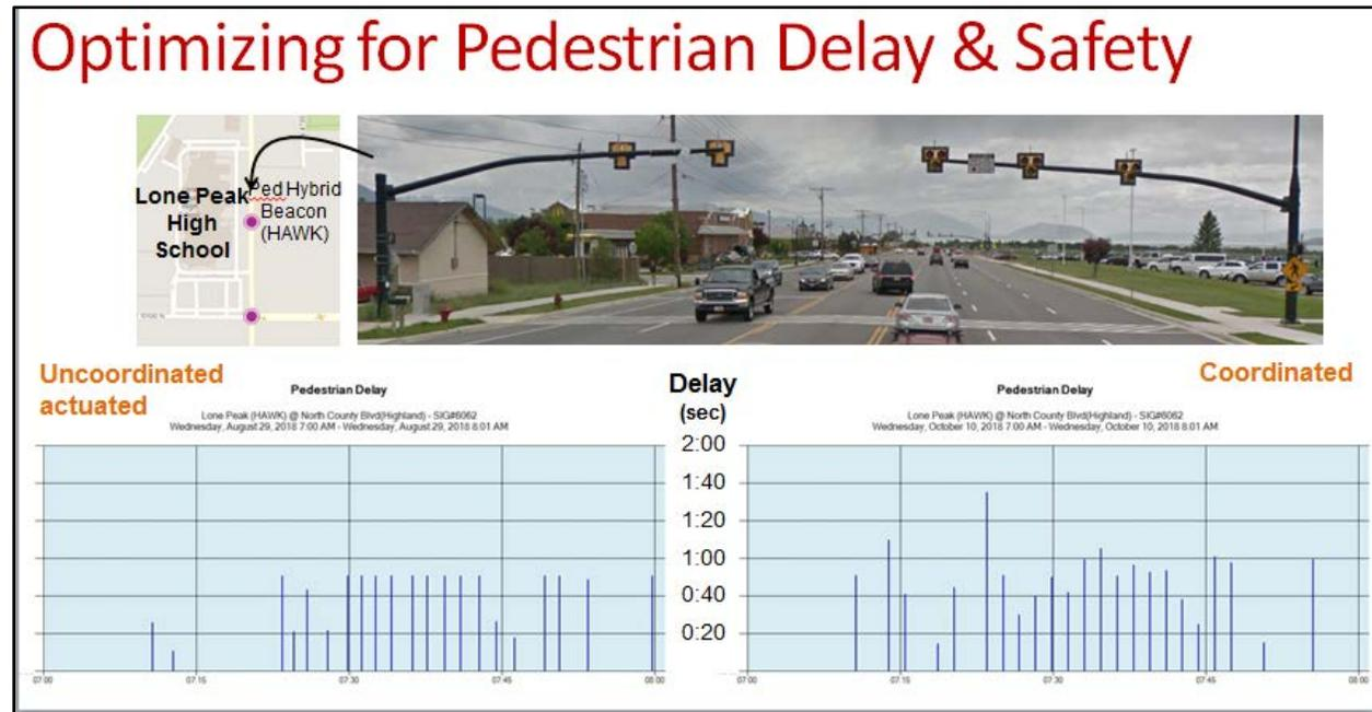
Figure 2.22 Changes in Pedestrian Delay When Adding Coordination
