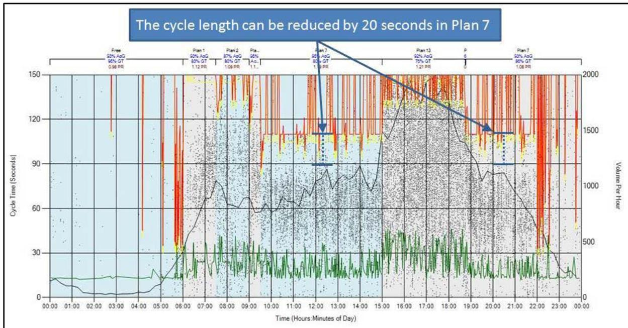
Figure 2.20 PCD Indicates Need for Lower Cycle Length - GDOT
