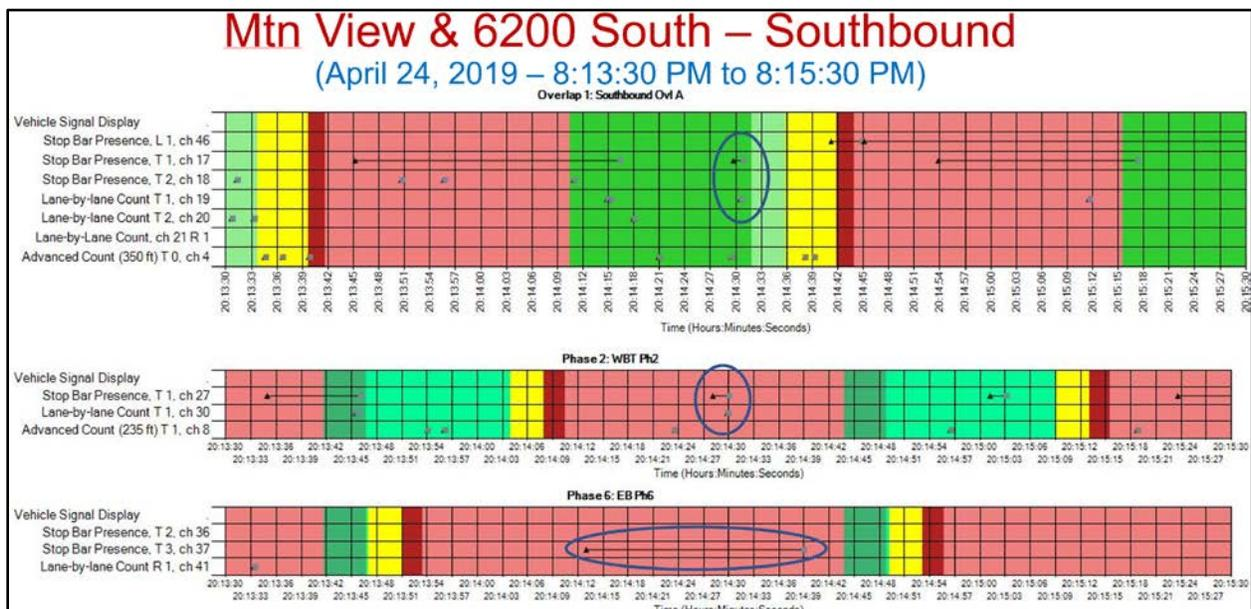
Figure 1.26 Timing and Actuation - Signal #7526 – Time range: 8:13:30 PM to 8:15:30 PM
