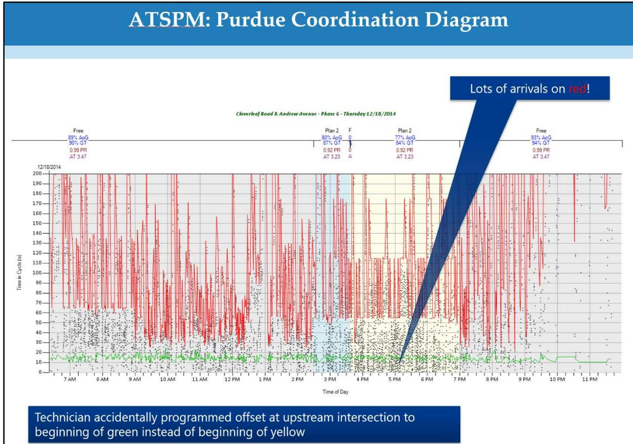
Figure 2.28 PCD Used to Identify Offset Concern (BEFORE) - PennDOT
