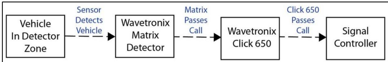
Figure 1.23 Detector call path explaining various points of potential latency
