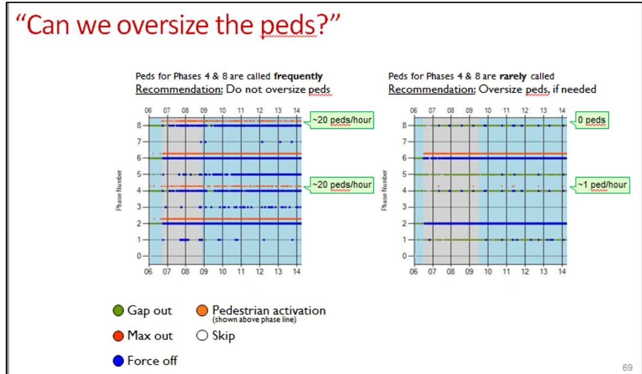
Figure 2.23 Evaluating if Pedestrian Times Can be Over-sized
