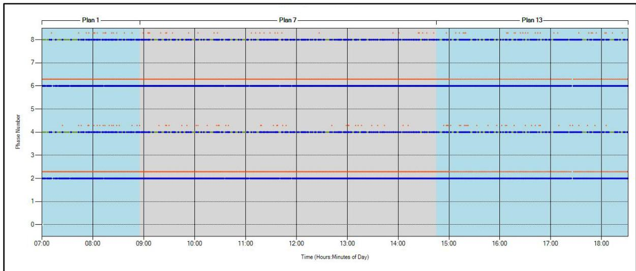
Figure 2.19 High Force Offs Indicate Need for Higher Cycle Length
