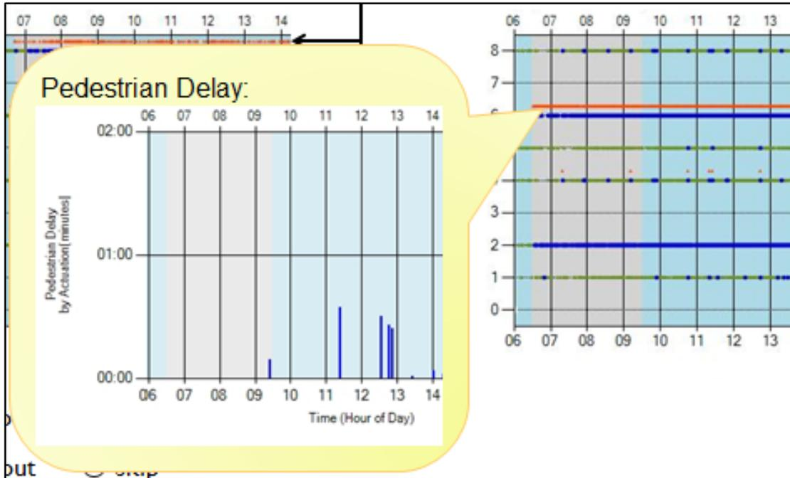
Figure 2.24 Pedestrian Delay Shows Pedestrian Actuations on Coordinated Phases
