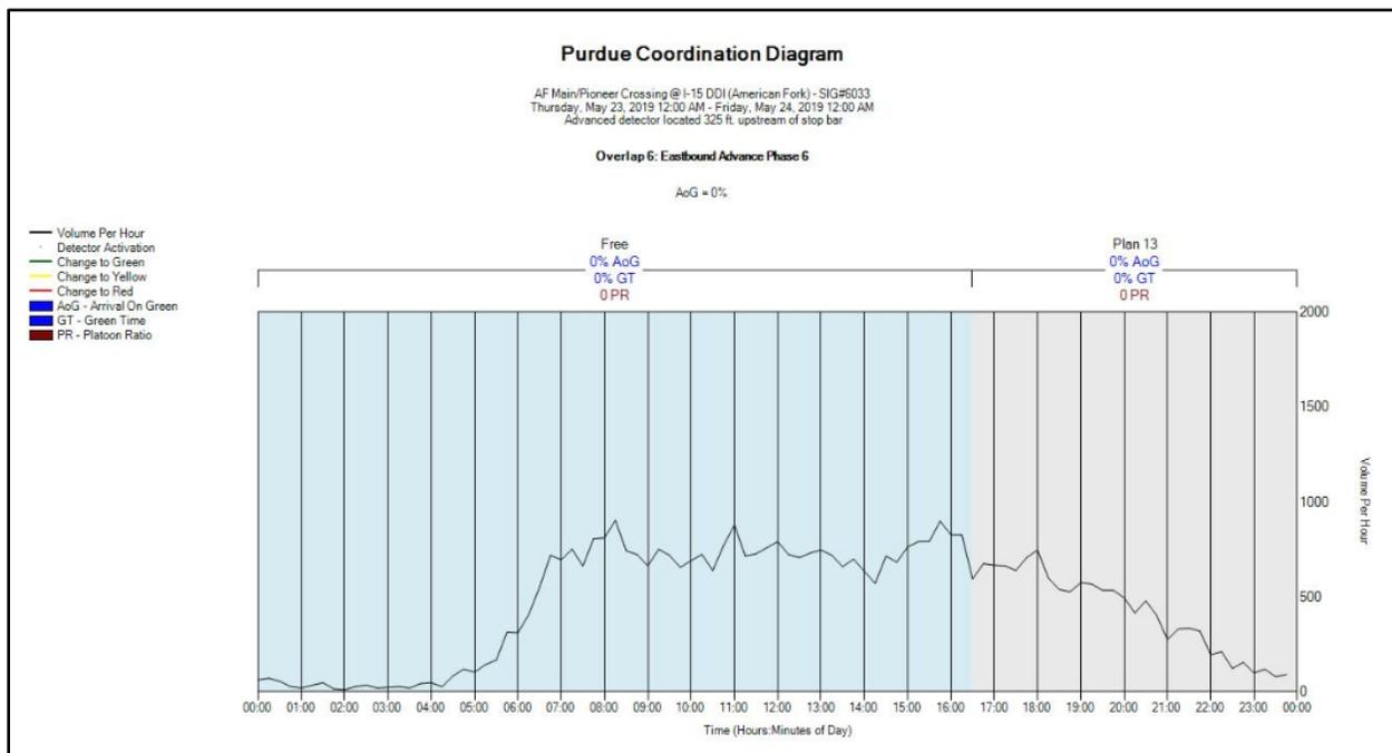
Figure 1.10 PCD with No Phase Data
