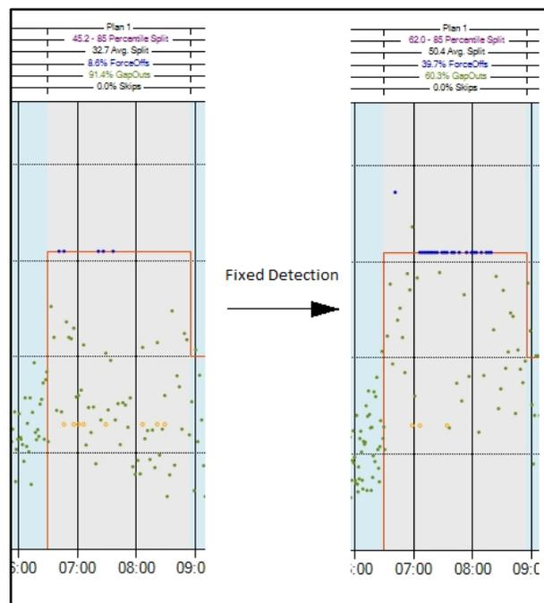
Figure 1.13 Split Monitor with Less Gap Outs
