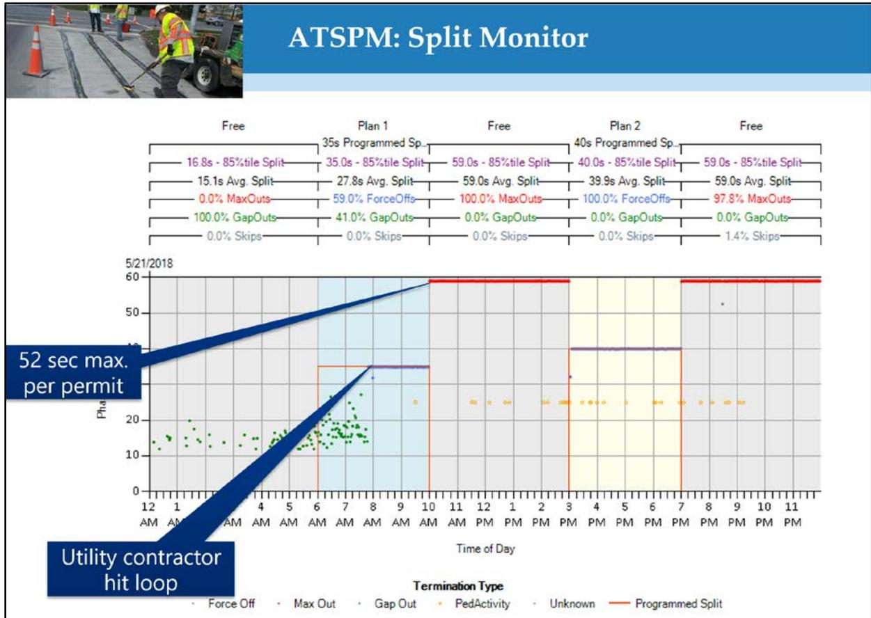
Figure 1.20 Detection Destroyed with Large Maximum Green Time – PennDOT
