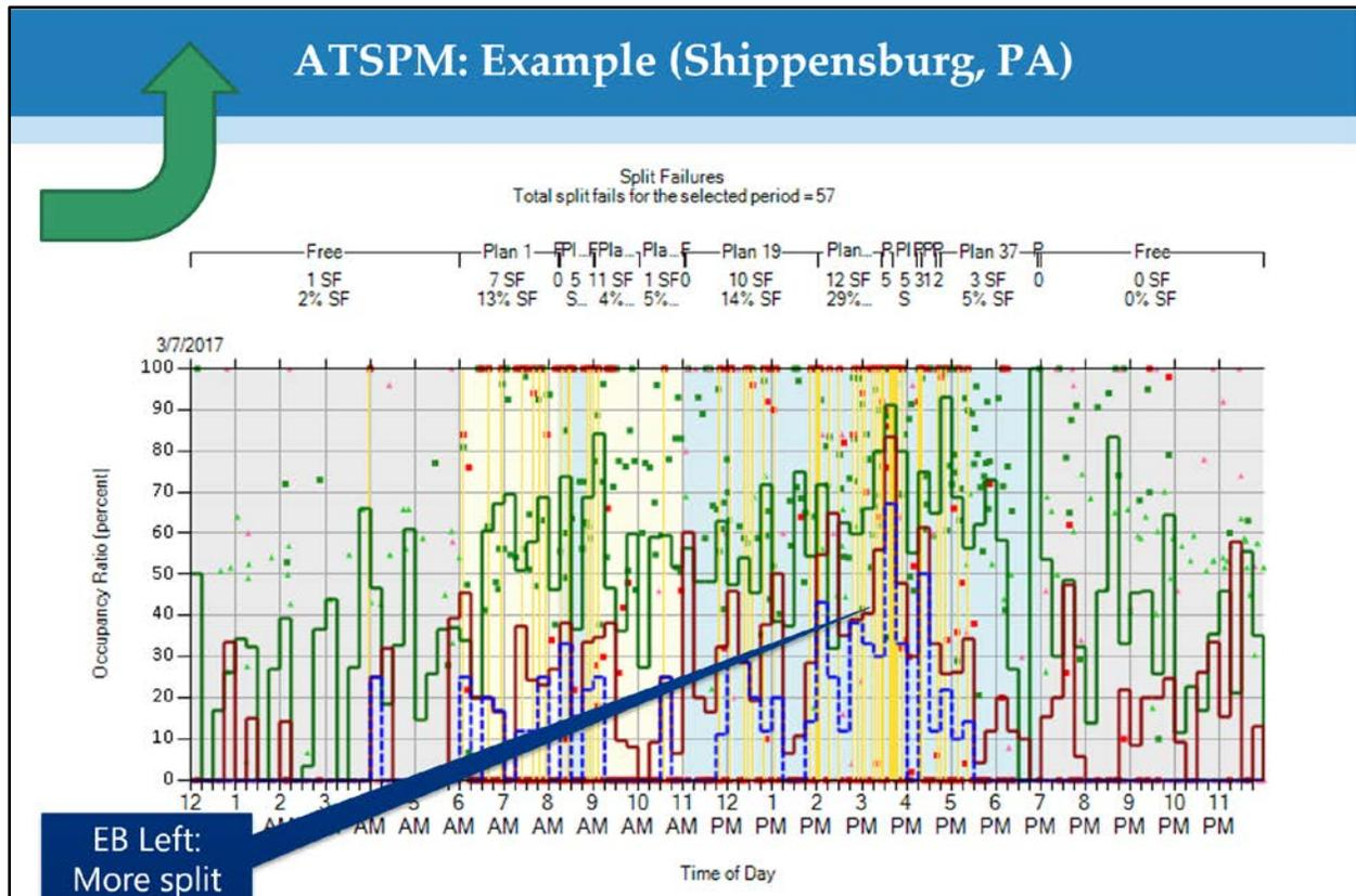
Figure 2.12 Purdue Split Fail Sequence Change Analysis (EB Left) - PennDOT
