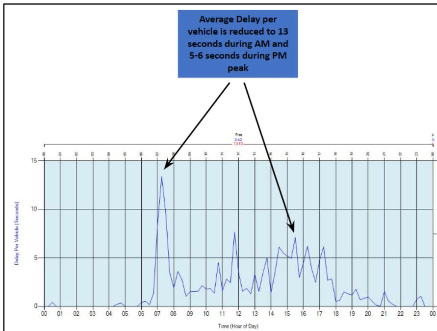
Figure 2.16 Approach Delay Chart after Changes - GDOT
