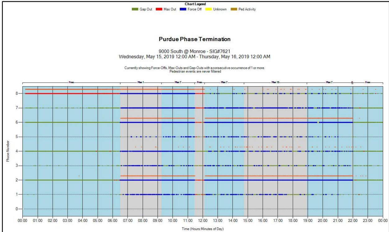
Figure 1.6 Stuck Pedestrian Button Causing Max Outs
