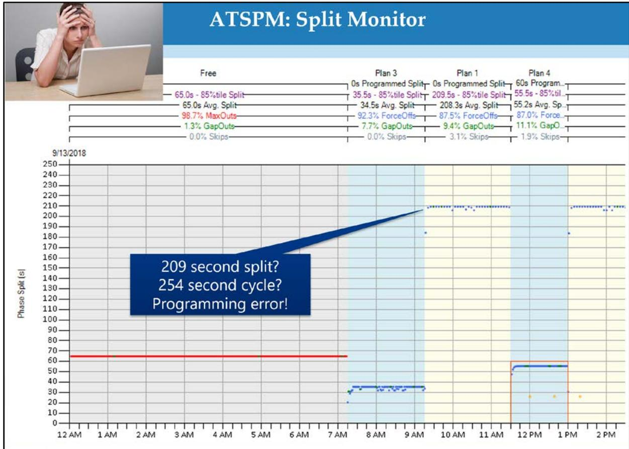
Figure 2.21 Incorrect Cycle Length Example - PennDOT
