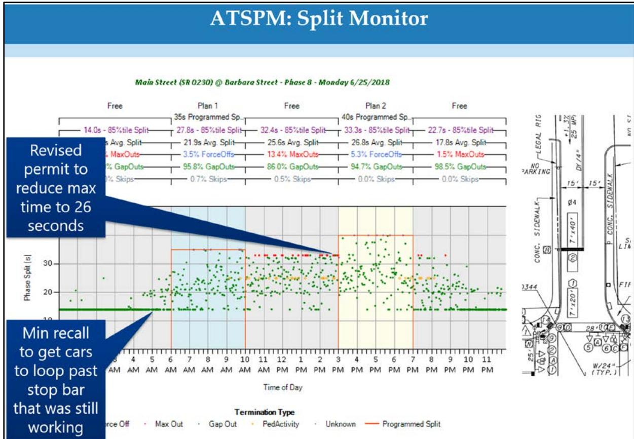
Figure 2.6 Split Monitor Example of Revising Permit with too much green time – PennDOT
