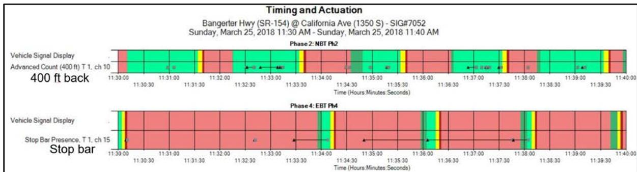
Figure 1.24 Timing and Actuation Metric - 10 minute window of analysis
