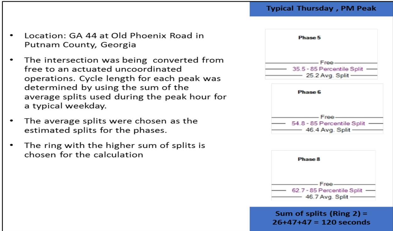
Figure 2.18 Coordination Cycle Length Analysis - GDOT
