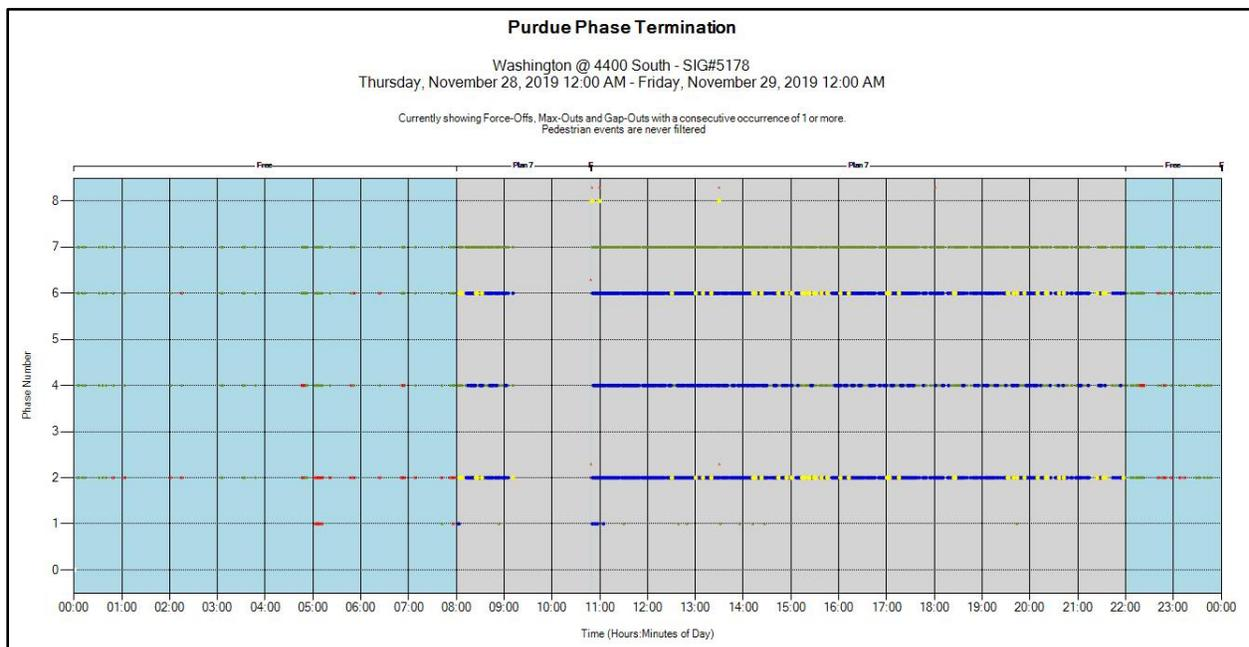
Figure 1.29 Purdue Phase Termination - Signal #5178 – November 29, 2019
