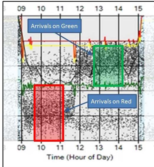
Figure 2.26 PCD Where Offset was corrected at 11:45
