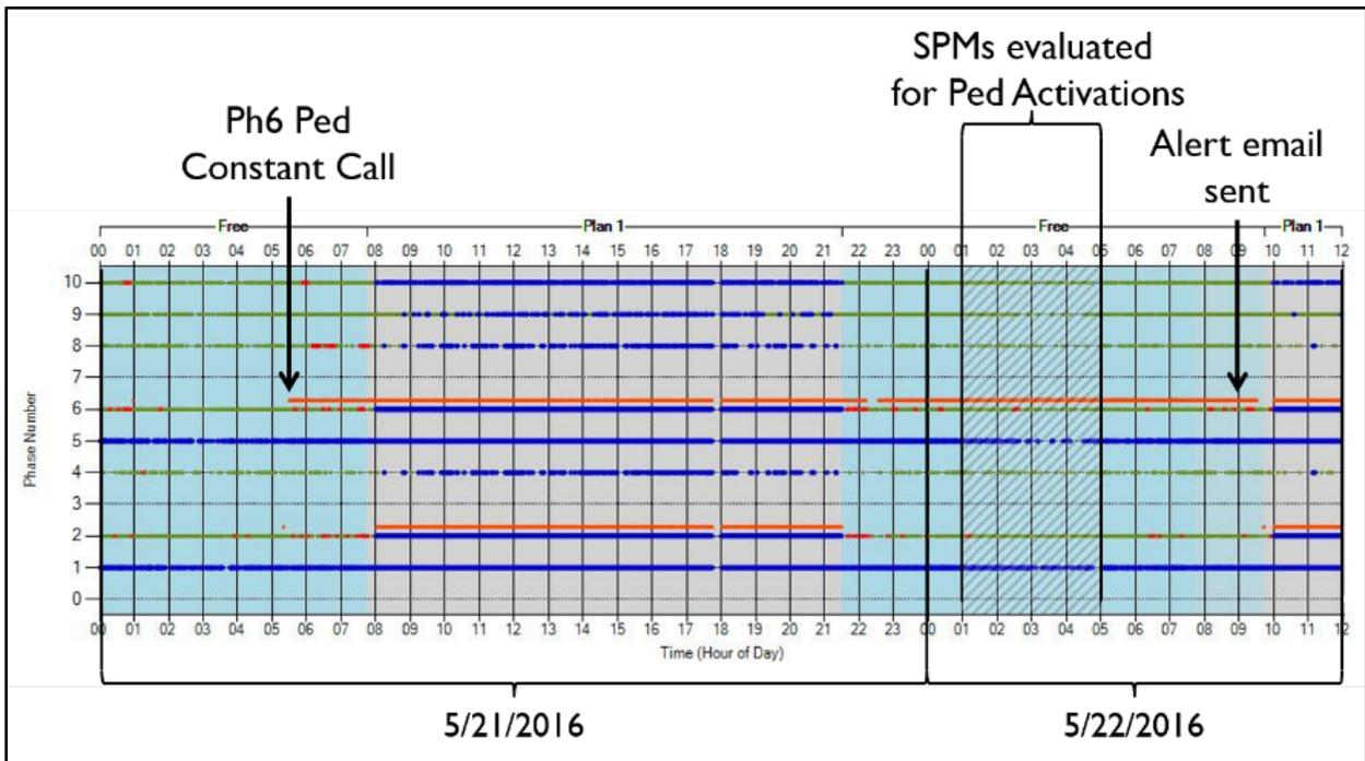
Figure 1.12 ATSPM Evaluation for High Pedestrian Activation Occurrences
