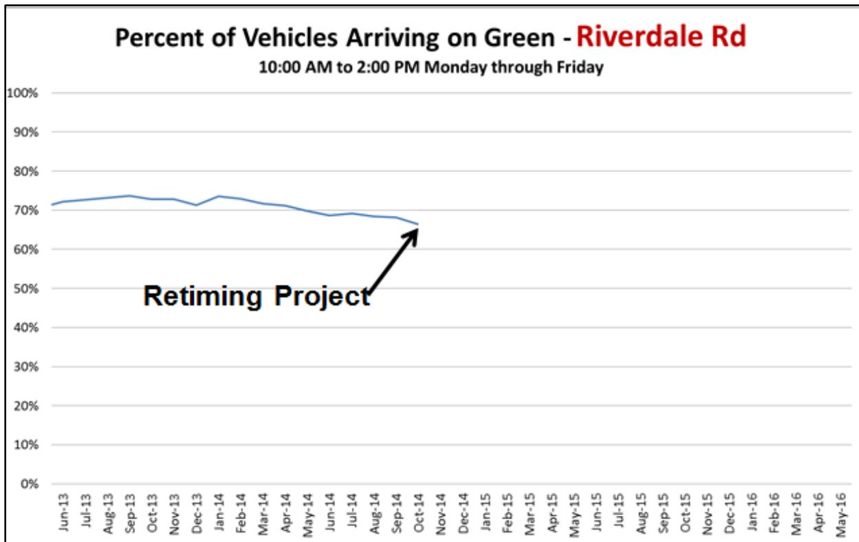
Figure 2.32 Degradation of AOG Triggers Coordination Optimization
